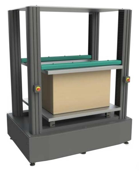
Floor-standing Box Compression machines with full computer control and precision AC servo drive system. Rigid 4-column load frame with lower platen mounted on 4 balanced load cells for improved accuracy and tolerance of uneven loading.
