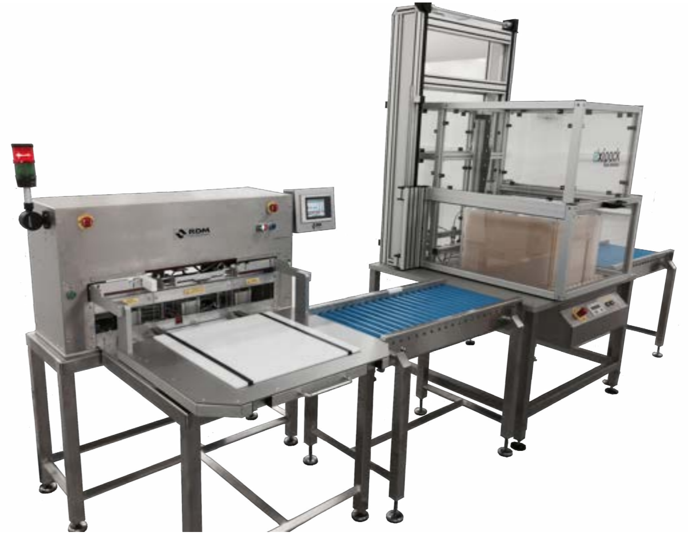
Customised HSX - 800 Heat Sealer, integrated with a Oxipack Leak tester.
